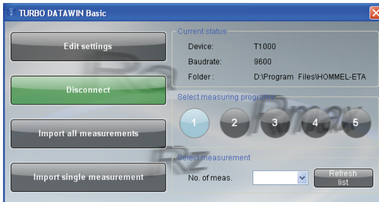
Figure 3-6: The connection between the PC and the measuring instrument has been established
