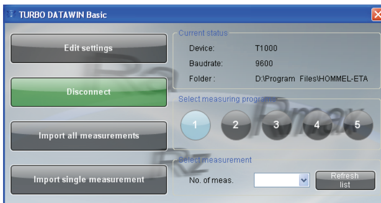
Figure 3-7: Performing the data import (T1000 in the example)
