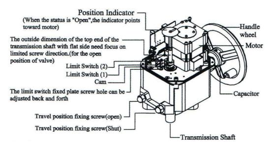
Cam Regulation for automatic operation works as in the previous cases; for Manual Operation please screw or unscrew the front travel position screws:
