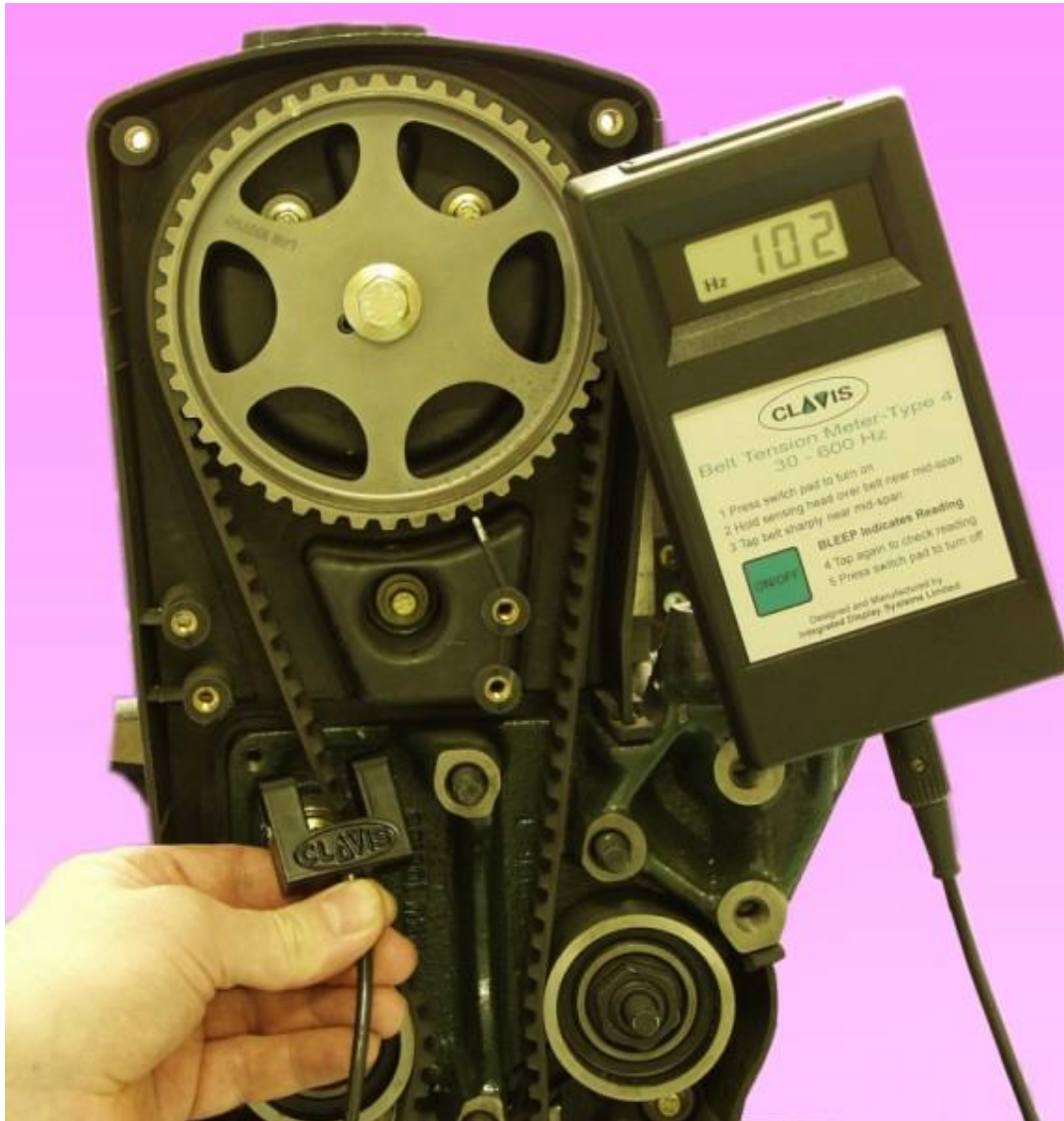
The CLAVIS hand held Belt Tension Meter (Type 4)
