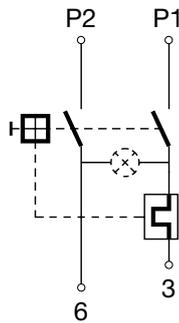
1 pole thermal overload protection, Shunt terminal
