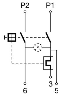
2 pole thermal overload protection
